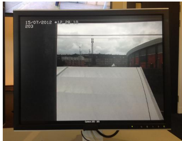
Figure 133: Blocked camera view. This particular example shows a temporary structure that was erected in front of a working camera
