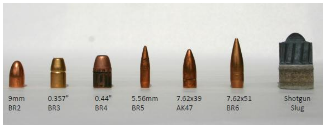
Figure 2 - The range of bullets used in BS EN 1063:2000
